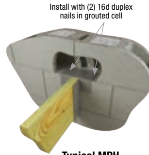
Typical MPH single-ply installation
