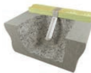
Alternate FA3 installation (concrete slab only)
