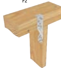
Typical TSP top plate installation (max nailing)
